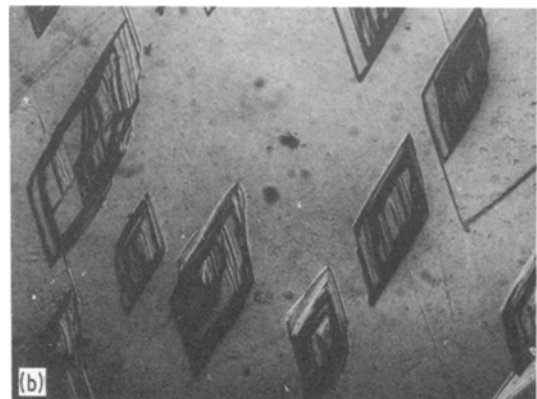
Figure 3(a) and (b) Etch patterns on matched cleavages etched in potassium hydroxide solution for 4 min ( \times 252 ).
