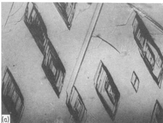
Figure 3(a) and (b) Etch patterns on matched cleavages etched in potassium hydroxide solution for 4 min ( \times 252 ).
